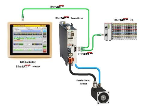
EtherCAT is a real-time Industrial Ethernet technology originally developed by Beckhoff Automation. It is industry standard and almost all the servo drive manufacturers have the EtherCAT option on their products.
