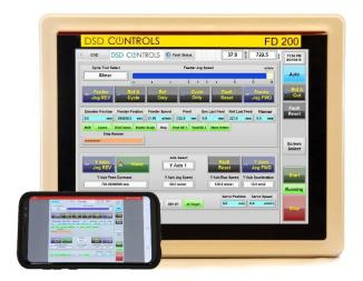
The controller is equipped with a remote success capability and by providing an EtherNET connection, our technician can access the controller anywhere in the world for troubleshooting, configuration, start-up, updates and upgrades.
